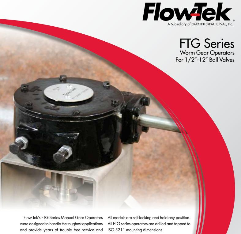
reliability. The FTG series Manual Gear Operators and provide years of trouble free service and reliability. The FTG series gear operators feature a ductile iron housing, aluminum bronze gear segment, one piece steel worm gear input shaft with tapered roller bearings on both ends. Adjustable travel stops provide precise adjustment in both open and closed positions. Housings are sealed and weather proof to fully isolate internal parts from atmospheric conditions.
